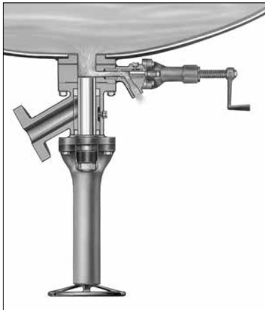
Fig. 2 - Drain Valve Open for Sample
