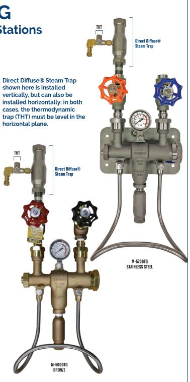
Maximum water temperature: 200°F (93°C) Optimum working pressure range: see chart at left (not to exceed 150 psi)
